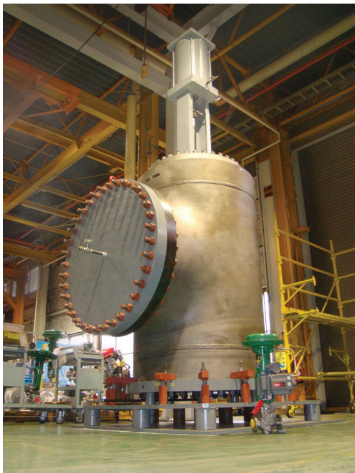
NPS 38 x 42 Fisher antisurge valve with ODV package next to a small NPS 1 Fisher easy-e valve for a size comparison
