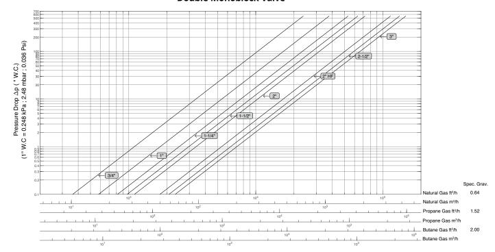
Notes: Flow curves are based on the following standard conditions: 5 psi (0.3 bar) inlet pressure and 68°F (20°C) fluid temperature. The Single and Monoblock Valve Flow Curves are based on Standard Seal constructions.
