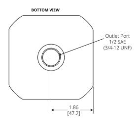
All dimensions are reference & nominal Metric [millimeter] equivalents are in brackets
