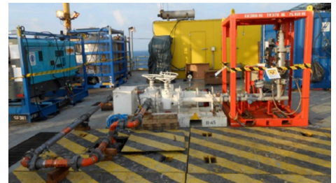
Image 1. The Roxar 2600 MPFM in use in field
