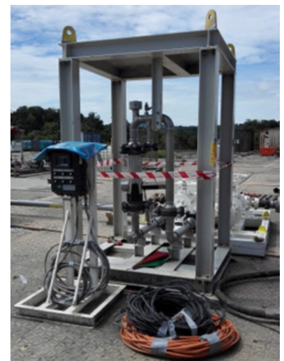
Image 1. The Roxar 2600 MPFM in skid arrangement in Papua New Guinea
