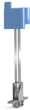
Five Rosemount Wireless Permasense ultrasonic thickness measuring sensors, mounted at strategic points around the header, helped determine the carbon steel header pipe wall was thinning at a rate of 2 mm (0.08-in.) per year.
