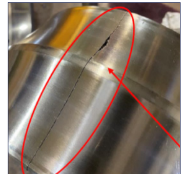
Full-width crack of the inner race of bearing.
