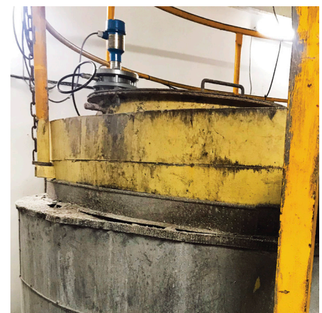
Image 2. The Rosemount 3408 features special Solid algorithm together with Smart Echo Supervision, which monitors the surface echo automatically and identifies which echoes are false dynamically
