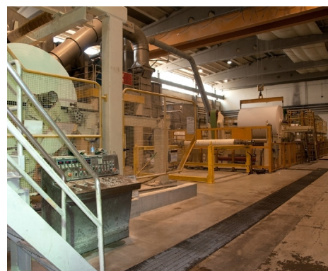
The continuous machine for texture paper production is the main steam consumer of the mill.
