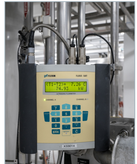
With the FLUXUS® G601 CA Energy, a temporary heat flow measurement can be set up in next to no time (i.e. thermal power measurement).
