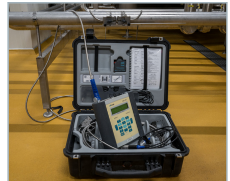
Compact in its case: the FLUXUS® G601 CA Energy ultrasonic measuring system.
