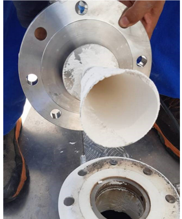
Prior to using the air purging feature, the Rosemount 5408 antenna is coated with flour
