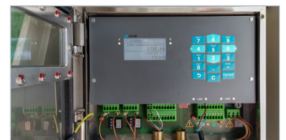
The stationary PIOX® S721 ultrasonic systems are used as measuring transmitters.
