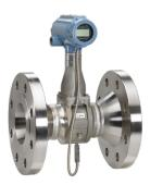
The Vortex flow meter product range is designed for utility and process applications. Features include the Adaptive Digital Signal Processing (ADSP) to provide immunity from vibration causing unstable or false flow readings and the robust design enables the sensor to be replaced without down-time. Additionally, input from an external HART® pressure transmitter provides temperature and pressure compensation, enabling compensated mass flow and corrected volume in steam and liquid applications.
