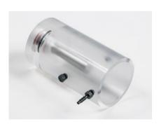
This specialized horn permits high-intensity sound to be applied to multiple samples without direct horn contact. 1.0" diameter only.
