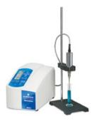
The support stand with stainless steel rod accommodates Branson's 40 kHz traditional converter. The converter holder supports the ultrasonic stack (converter and microtip) and is adjusted easily to properly position the microtip in the sample.
