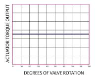
Torque output of the rotary vane actuator remains constant throughout the full rotation of the valve. This ensures that your specified safety factor will not be jeopardized at different positions during the valve stroke. Constant torque output is an especially important feature in the following applications:
