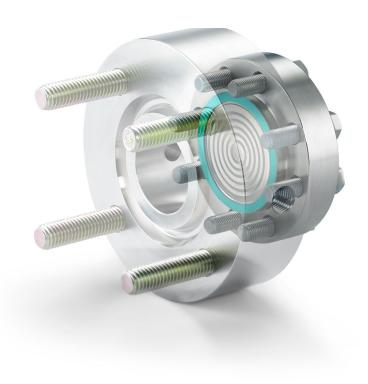
Many pressure instrument installations rely on diaphragm seals to keep the process fluid where it belongs, while delivering accurate and repeatable pressure measurements across a wide variety of operating conditions. They can support gauge, absolute or differential pressure (DP), which extends potential use to flow and level measurements and can serve as remote seals where their physical size fits the application.
