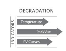
• PeakVue technology recognizes degradation ahead of PV Curves (a comparison of pressure to the volume of gas) and before temperatures increase.
