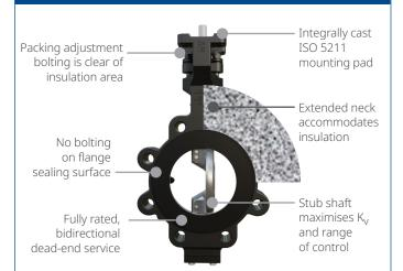
**Simplify your valve assets** with a solution designed to suit your chemical facility. The lug style valve provides full rated, bidirectional dead-end service with an uninterrupted flange sealing surface in compliance with EN 12569. The valve is designed to NAMUR NE 167, ISO and EN specifications with PED and CE certifications as standard.
