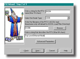
trollers. Above this communication layer are a group of applications known as Bristol OpenBSI Utilities. These client utilities communicate through the server to collect and manage data from the controllers and RTUs, generate files based on collected historical data, collect alarms, and monitor and control OpenBSI communications.
