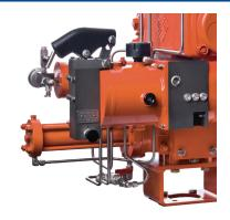
Corrosion resistant materials ensure longevity. The control enclosure, hydraulic manifold and hand pump are constructed from marine grade aluminum with stainless steel trim.
