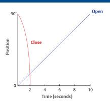
Fast-closing or precise speed control is obtained through field-adjustable flow control valves to meet application requirements.
