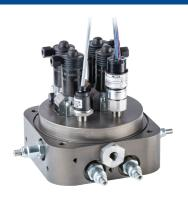
Solenoids, speed controls, pressure transducers and pressure switches are integrated in a compact manifold block eliminating external tubing and connections.
