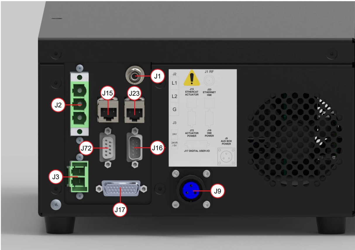
Figure 4.6 GSX Power Supply Cable Interface Points
