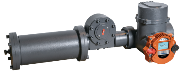
Figure 2: The Bettis RTS low power, all electric actuator can be ordered with a fail-safe spring and mounted on quarter turn or linear valves. The intelligent controller provides embedded PID and programmable stroke functionality.
