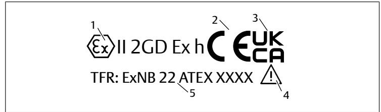
Fig. 3: Name plate for mechanical explosion protection
