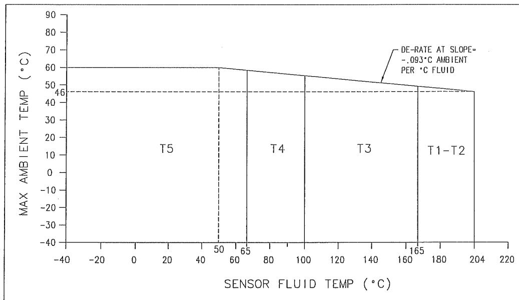
Note: Use the above graph to determine the temperature class for a given fluid and ambient temperature. The maximum surface temperature T for dust is as follows: T5: 95 °C, T4: 130 °C, T3: 195 °C, T2: to T1: 234 °C.
