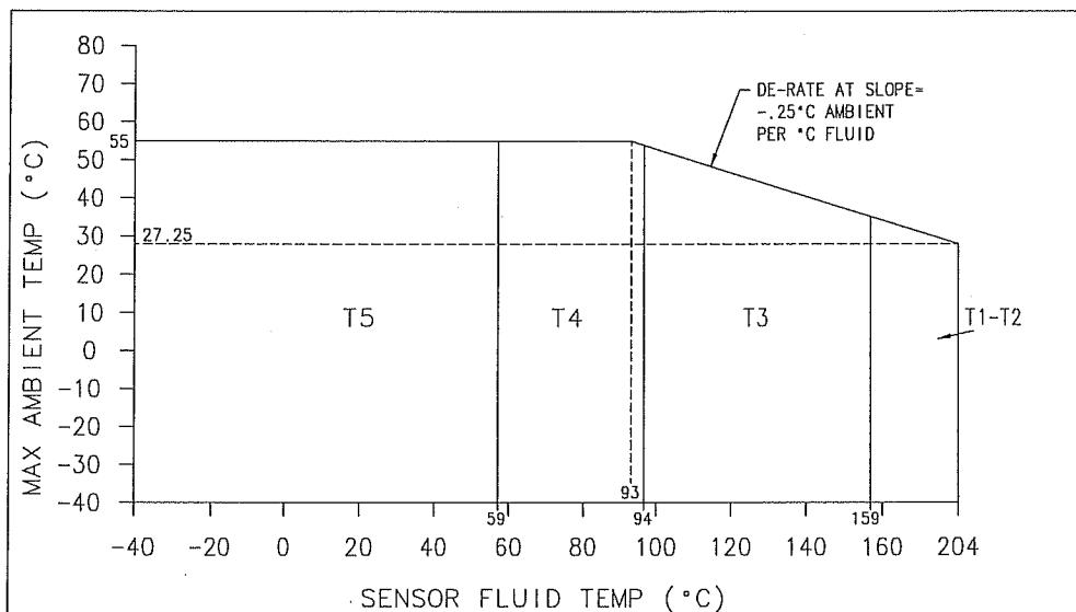
Note: Use the above graph to determine the temperature class for a given fluid and ambient temperature. The maximum surface temperature T for dust is as follows: T5: 95 °C, T4: 130 °C, T3: 195 °C, T2: to T1: 240 °C.
