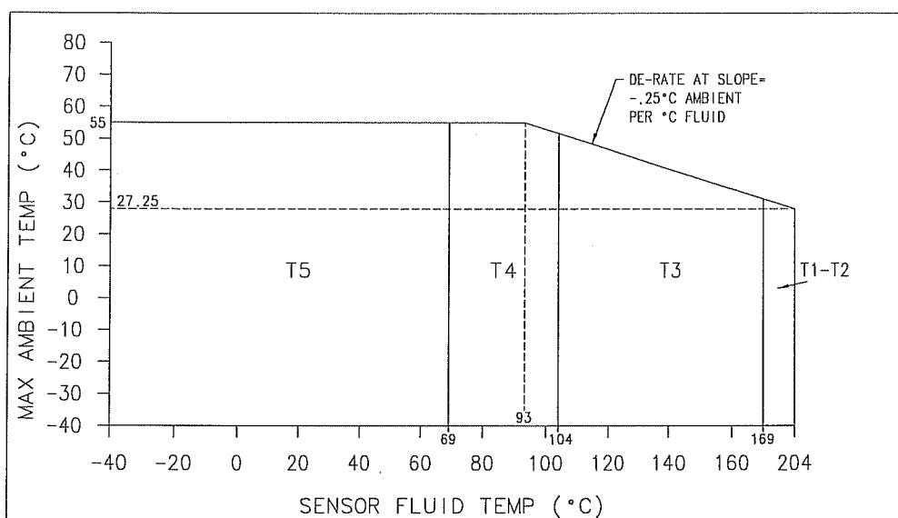
Note: Use the above graph to determine the temperature class for a given fluid and ambient temperature. The maximum surface temperature T for dust is as follows: T5: 95 °C, T4: 130 °C, T3: 195 °C, T2: to T1: 230 °C.
