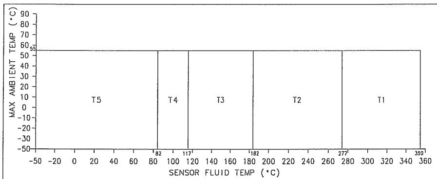
Note: Use the above graph to determine the temperature class for a given fluid and ambient temperature. The maximum surface temperature T for dust is as follows: T5: 95 °C, T4: 130 °C, T3: 195 °C, T2: 290 °C and T1: 363 °C.
