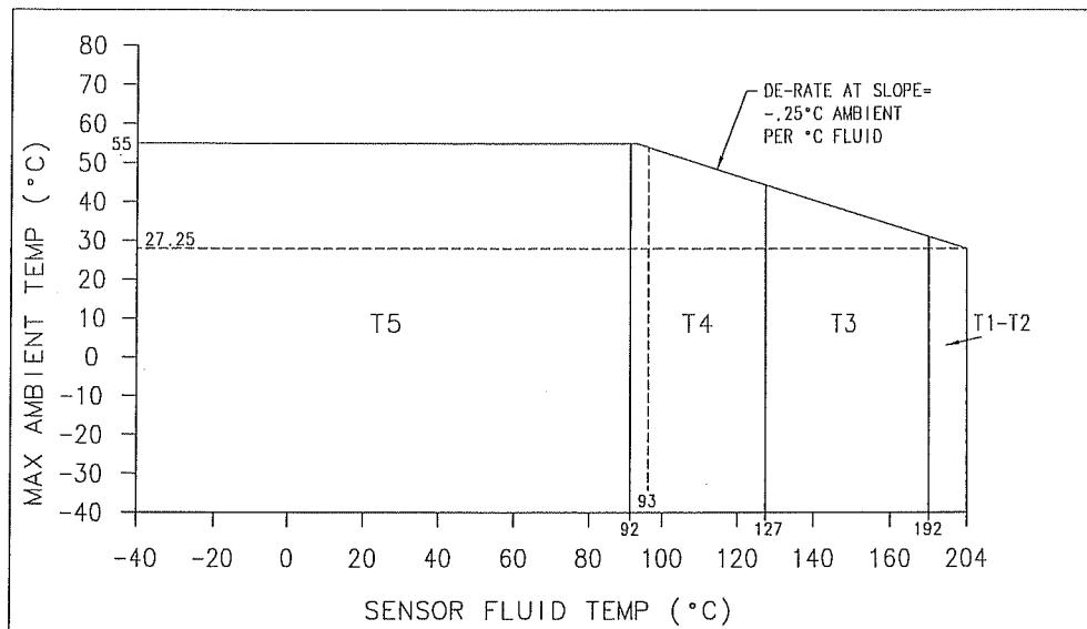
Note: Use the above graph to determine the temperature class for a given fluid and ambient temperature. The maximum surface temperature  $T$  for dust is as follows: T5: 95 °C, T4: 130 °C, T3: 195 °C, T2: to T1: 207 °C.
