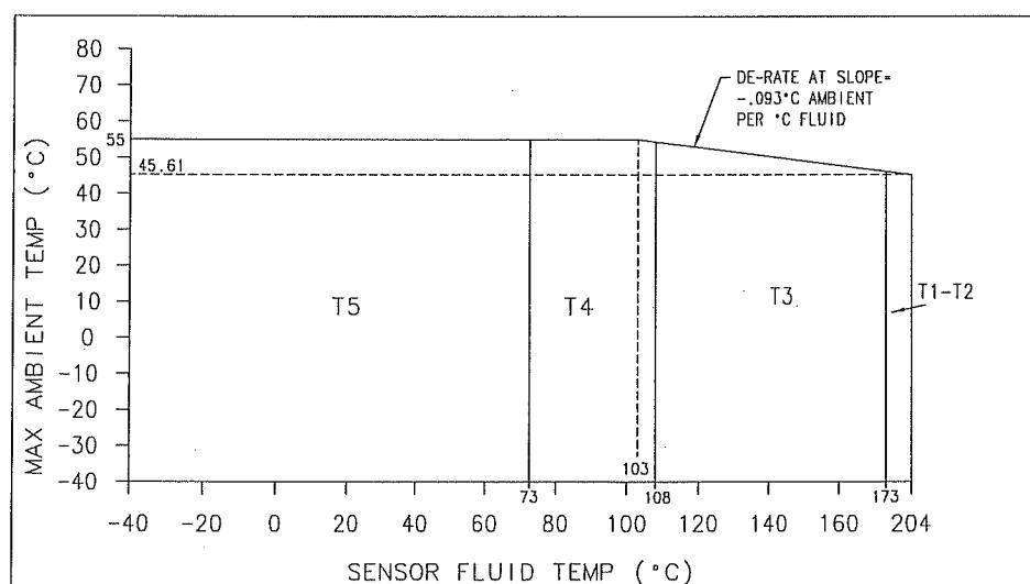
Note: Use the above graph to determine the temperature class for a given fluid and ambient temperature. The maximum surface temperature T for dust is as follows: T5: 95 °C, T4: 130 °C, T3: 195 °C, T2: to T1: 226 °C.
