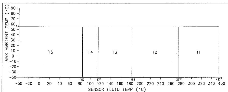
Note: Use the above graph to determine the temperature class for a given fluid and ambient temperature. The maximum surface temperature T for dust is as follows: T5: 95 °C, T4: 130 °C, T3: 195 °C, T2: 290 °C and T1: 440 °C.
