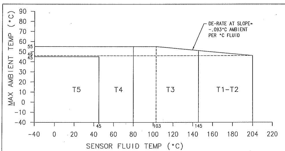
Note: Use the above graph to determine the temperature class for a given fluid and ambient temperature. The maximum surface temperature T for dust is as follows: T5: 95 °C, T4: 130 °C, T3: 195 °C, T2: to T1: 254 °C.
