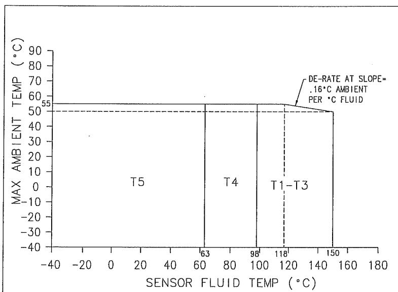
Note: Use the above graph to determine the temperature class for a given fluid and ambient temperature. The maximum surface temperature T for dust is as follows: T5: 95 °C, T4: 130 °C, T3: to T1: 182 °C.
