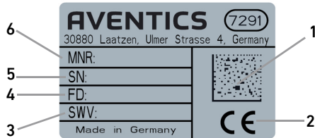
Fig. 1: Type plate of the Joystick Type 531
