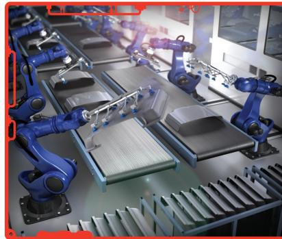
valves can hold vacuum towards the gripper function to keep the gripped object in position for a time until the vacuum resumes.
