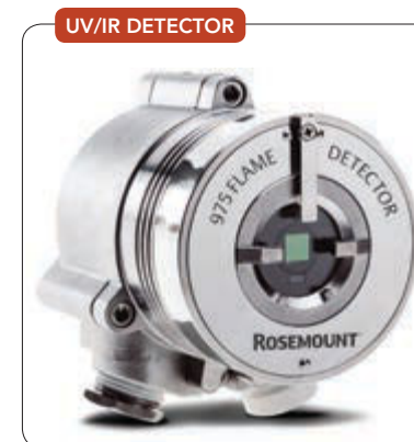
Figure 1. This instrument must detect flames on both bands to trigger an alarm.
