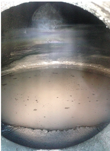
Fig. 3a. Sand but no beach—looking in an inspection port shows a characteristic build-up of sand and emulsified water that accumulates in the separator.
