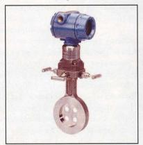
ble measurement and provide 0.5% accuracy with two diameters of straight piperun. It works with a Model 3051S transmitter and software to form a 3051SFC flowmeter. The flowmeter is suitable for gas and steam applications where a compensated flow output is required.
