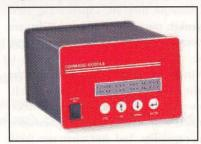
All functions can be programmed through the integrated keypad using menu-driven software, or set up via RS-232 or HTML/TelNet interfaces.
