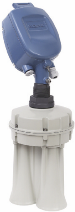
Emerson's Rosemount 5708 3D Solids Scanner supports the continuous analysis of product flow and movement by dividing a large vessel into as many as 99 smaller, virtual sections
