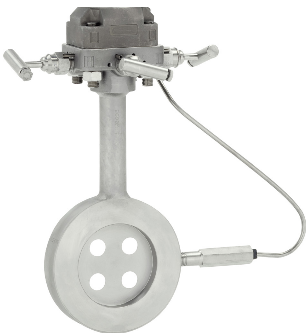
Figure 2. A conditioning orifice with multiple holes reduces the need for long straight pipe runs upstream and downstream.
