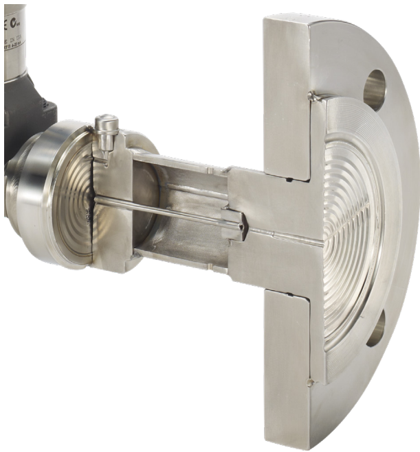
Figure 3. As this cut-away unit shows, the external diaphragm is exposed to the cold liquid but does not allow it to reach the internal diaphragm, so the reading response is not slowed.
