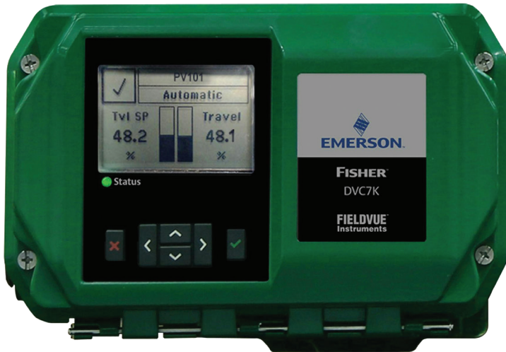
◀ Figure 3: A graphical interface, LED status light, along with easy-to-use buttons, can be an invaluable aid to technicians, helping them quickly resolve problems. (Fisher FIELDVUE DVC7K shown)
