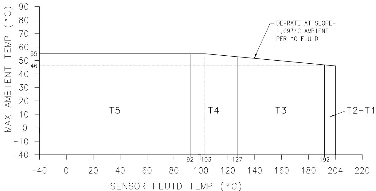
Note: Use the above graph to determine the temperature class for a given fluid and ambient temperature.
