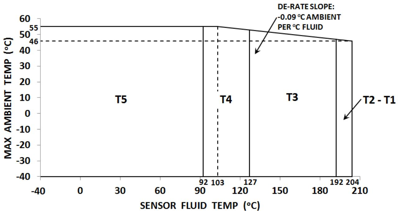
Note: Use the above graph to determine the temperature class for a given fluid and ambient temperature.
