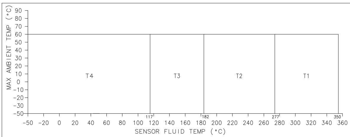
Note: Use the above graph to determine the temperature class for a given fluid and ambient temperature.
