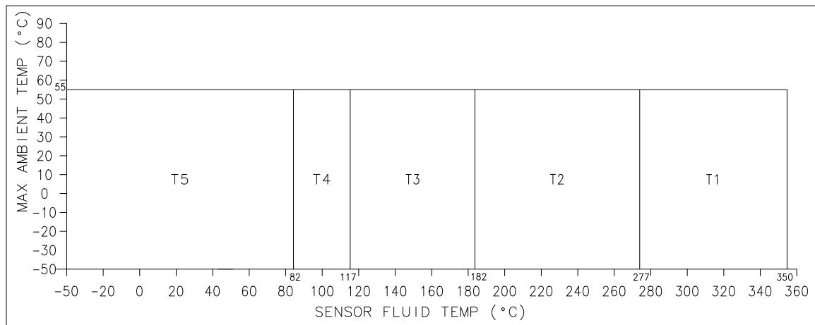
Note: Use the above graph to determine the temperature class for a given fluid and ambient temperature.
