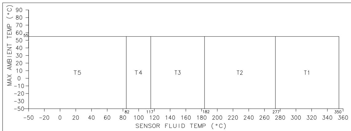
Note 1: Use the above graph to determine the temperature class for a given fluid and ambient temperature.
