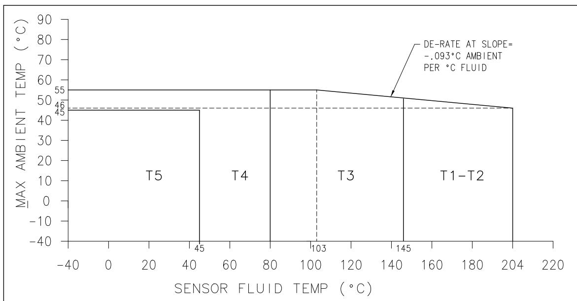
Note 1: Use the above graph to determine the temperature class for a given fluid and ambient temperature.
