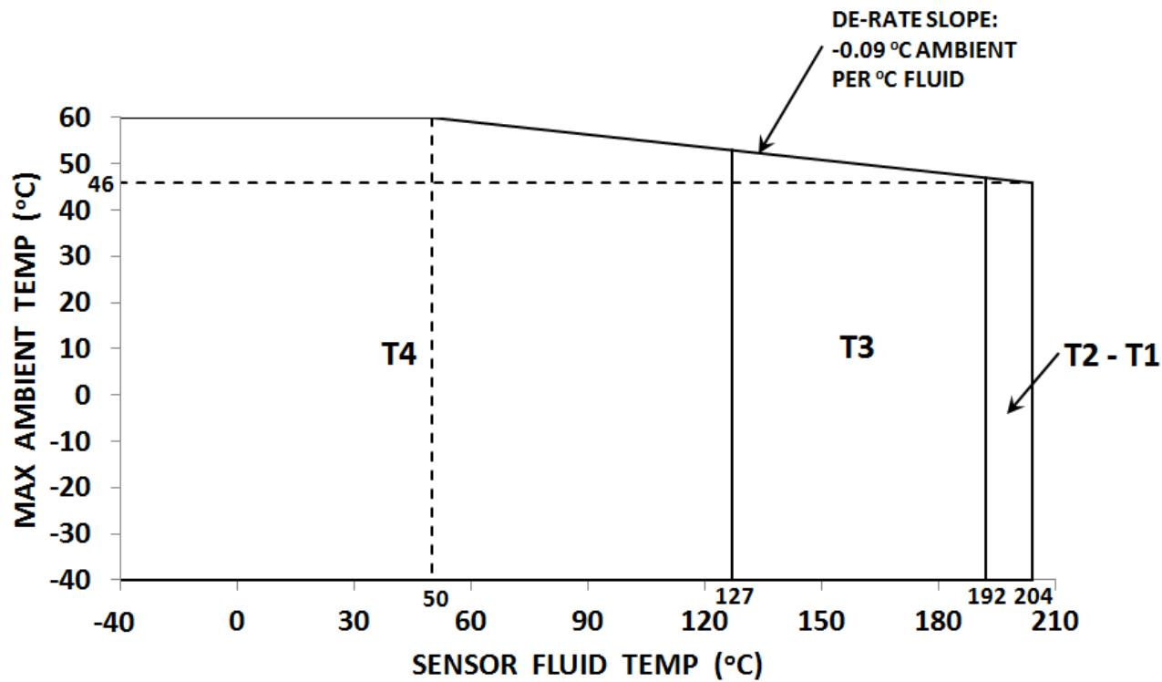
Note 1: Use the above graph to determine the temperature class for a given fluid and ambient temperature.
