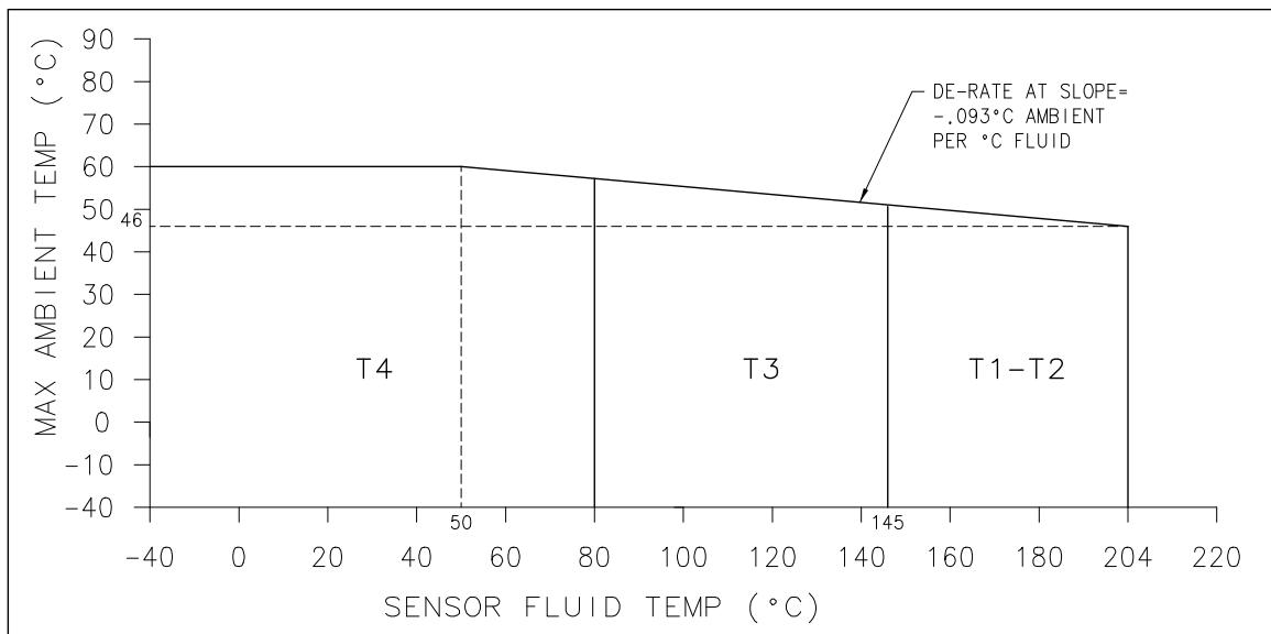
Note 1: Use the above graph to determine the temperature class for a given fluid and ambient temperature.
