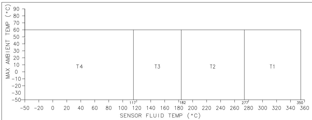
Note 1: Use the above graph to determine the temperature class for a given fluid and ambient temperature.
