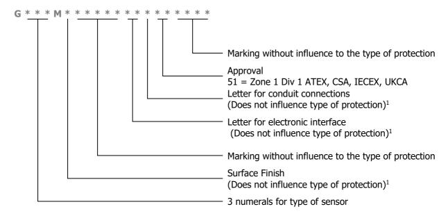
Below are examples of different Gxxx sensor configurations: (detailed in Installation Instruction EB-2009779)
