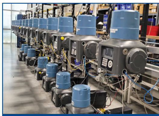
Figure 2 Design verification testing of the Rosemount 470XA at the Houston, Texas factory.
