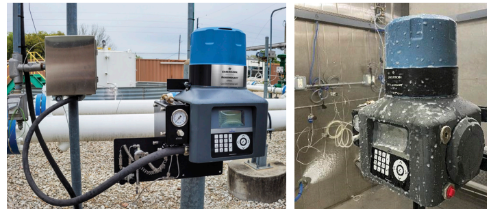
Figure 4 Rosemount prototypes in field testing (left) and cold temperature soak environment chamber testing (right).
