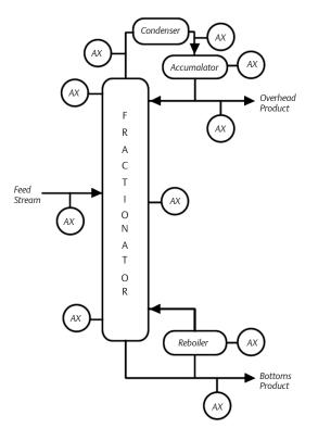
This is due to the fact that the tower separates by boiling point so if the concentration of one compound remains low, all the compounds that boil higher (or lower for the bottoms stream) will also be kept low. This compound is often referred to as the "key" compound the light key and heavy key. If these are minimized, all the other impurities are also minimized.
