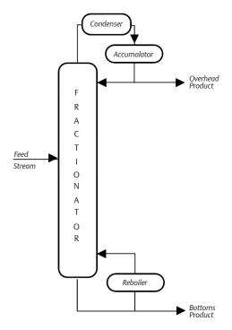
As the gases leave the top of the tower, they are cooled in a condenser, collected in an accumulator and then exit as the overhead product. To further increase the purity of the overhead stream, some of it is recycled (called reflux) for additional processing. The higher the reflux ratio, the purer the overhead product becomes.
