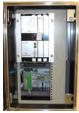
Figure 4-4: A6500MS in a compact wall-mount enclosure
