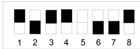
Figure 4.11 Type 1 DIP Switch Marked “OPEN” on Top of Switch, Default Settings
