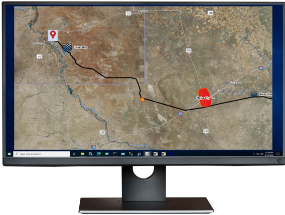
Figure 2. Advanced software with GIS capabilities provides control room operators with a clear view of a potential leak point.
