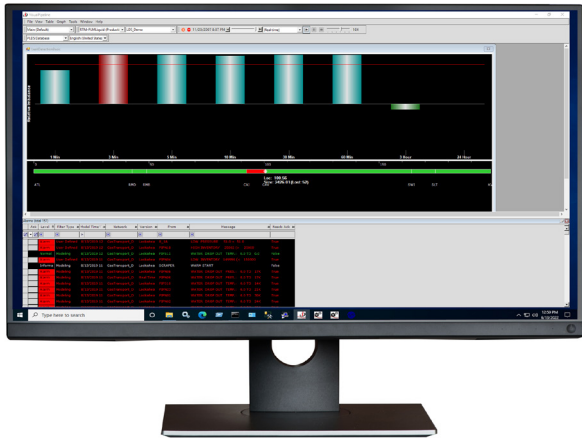
Figure 3. Emerson's PipelineManager software uses statistical analysis and filtering techniques to ensure leaks can be quickly identified and localised.
