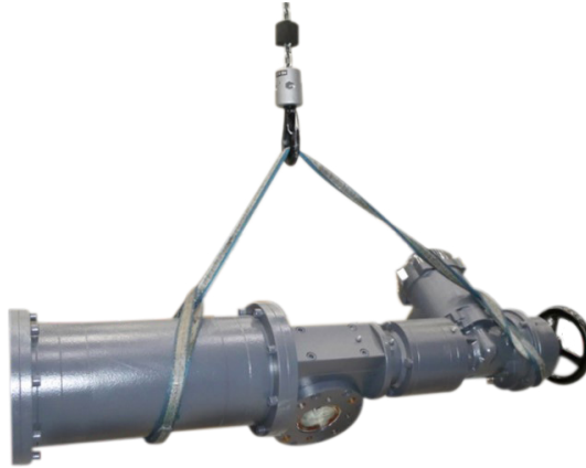
Figure 9. Proper Hoisting Technique 1
