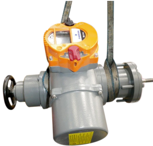
Figure 10. Proper Hoisting Technique 2
