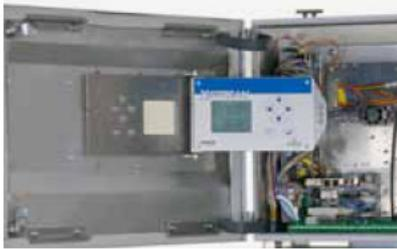
Interior view, showing 2 NDIR benches in an unheated upper compartment, a heated box option in the lower compartment, I/O boards.
