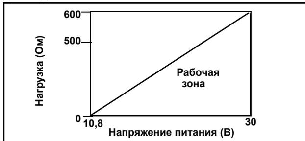
$$R_{\text{макс.}} = 31,25 (V_{\text{ps}} - 10,8)$$
