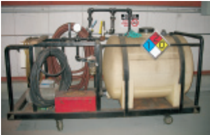
8. Portable wash skid cleans combined-cycle turbine compressors semiannually, peaker compressors annually
