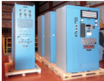
13. Speedtronic Mark II control cabinets rest on skids awaiting a buyer
