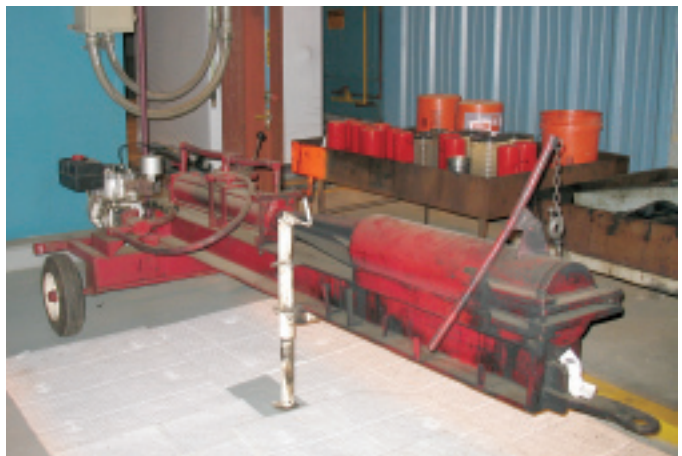
10. Lube-oil filters took up too much room in the dumpster for wastes requiring special handling, so plant personnel made a special compactor to reduce both volume and disposal cost
