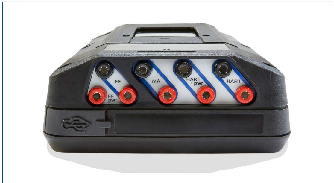
Connecting to loop power on the AMS Trex unit is simple and intuitive for both HART and FOUNDATION Fieldbus devices.
